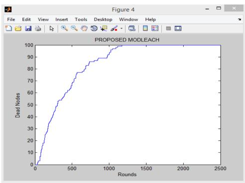
Figure 4.2 Dead nodes Vs No of Rounds for proposed MODLEACH protocol
