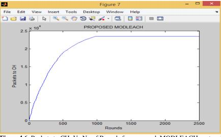
Figure 4.6 Packets to CH Vs No of Rounds for proposed MODLEACH protocol
