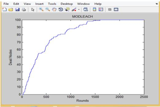
Figure4.1 Dead nodes Vs No of Rounds for MODLEACH protocol
